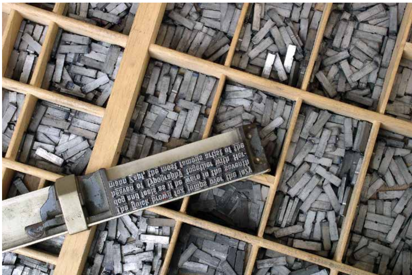
Letters of metal type allocated according to compartment, for each letter of the alphabet. A composer's stick is also shown, in which the letters are brought together to form words and sentences, ready for printing.
